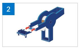
Remove the label and pop off the carrier's end clasp
