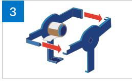
Undo the three snaps and pull the carrier apart – it will take a little force to separate the pieces
