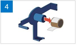
Remove the core from the carrier (separate the remaining wristband(s) from the core)
